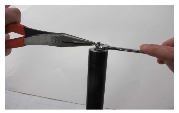
4) Use 5/16" wrench to turn nut, tightening the nut will adjust the tension and remove play in the shaft. Loosening the nut will allow more space between ferrule and shaft for less resistance when adjusting paddle height.
